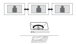
■ To enlarge or reduce the aspect ratio of the picture, press the button on the remote control to select Normal, 16:9, or Zoom (if available for the video source you're using).
