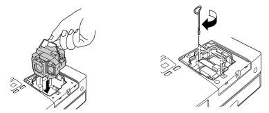
7. To replace the lamp cover, slide it into position, then tighten the screw. (The projector won't work if the lamp cover is loose.)
