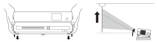
If the image is horizontally tilted, you can turn the feet to level it.
