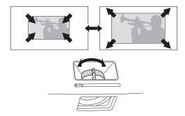
■ Rotate the focus ring to sharpen the picture.
